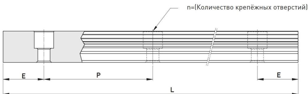
$$L = (n - 1) \times P + 2 \times E \quad \dots \dots \dots \Phi.2.2$$
