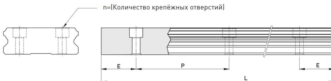
$$L = (n - 1) \times P + 2 \times E \quad \dots \dots \dots \quad \Phi.2.3$$
