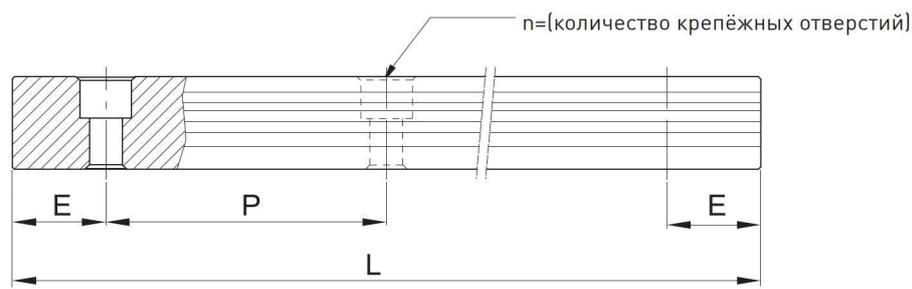
$$L = (n - 1) \times P + 2 \times E \dots\dots\dots \Phi.2.1$$
