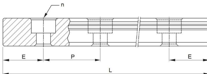
$$L = (n - 1) \times P + 2 \times E \quad \dots \quad \Phi.2.4$$
