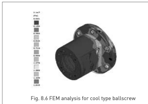
Fig. 8.6 FEM analysis for cool type ballscrew
