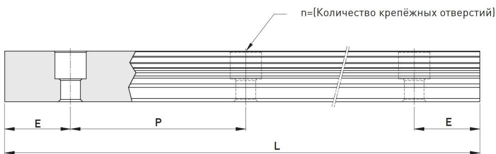
$$L = (n-1) \times P + 2 \times E \quad \dots \dots \dots \Phi.2.2$$
